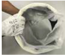
5. Feed the inner part of the new bag through the holder until it reaches the lower edge.
