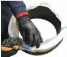
4. Cut and remove the closing clips from the previous LONGOPAC®.
